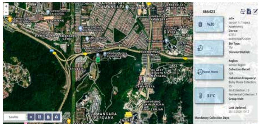
The system dashboard showing the level of the waste in the bin
