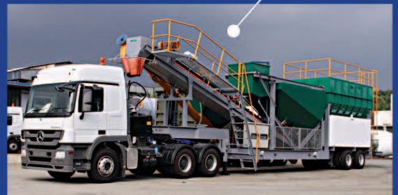
Buffulo Mobile Batching Plant Uses JOST Landing Gear & TTK Trailer Component
